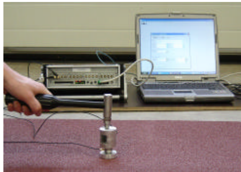
Figure A.20: Measurement system for mechanical impedance developed by M+P (The narrow part on top of the ground plate is the force transducer; the upper-part being struck by the impedance hammer comprises an accelerometer and its housing)
