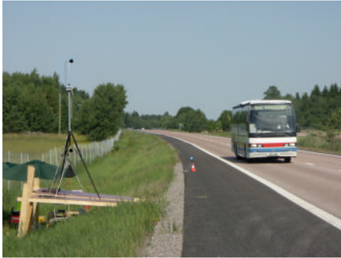
Figure 6.11: The low (1.2 m) and high (3.5 m) microphone positions used for the SPB measurements on the E18, Sweden. This is the section with double-layer porous asphalt measured when it was two years old. Note that the photo is highly zoomed; in reality the road at the site is totally horizontal and straight.
